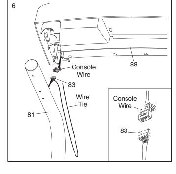
Set the Console (88) on the Handrails (80, 81). Start four M4.2 x 19mm Screws (6), two M5 x 16mm Screws (8), and two M5 Star Washers (9) into the Console as shown. Then, tighten all six Screws.
